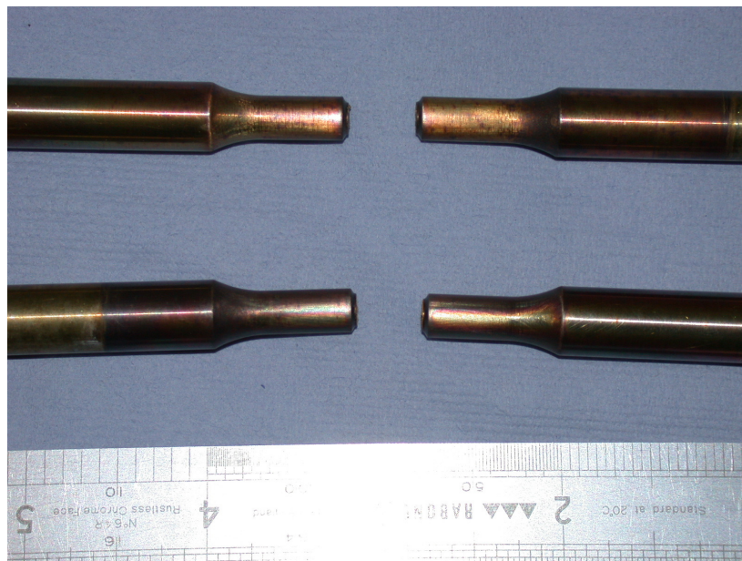
Fig. 3: Testpieces 7 & 8 (neat solution ) after exposure
