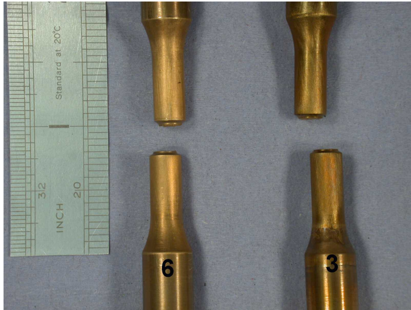
Fig. 2: Testpieces 3 (potable water) and 6 (diluted solution) after exposure
